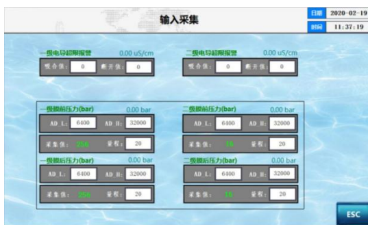
Conductivity alarm setting / 4-20ma input calibration
